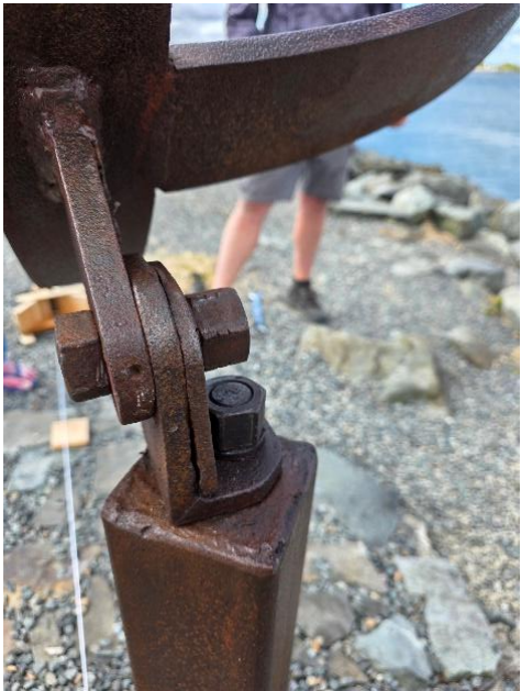
Rusted altitude and azimuth bolts that JJ had to loosen.
